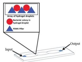
Figure 8: Design in the microfluidic device mimicking the tortuous flow of blood as in venous stasis cases
