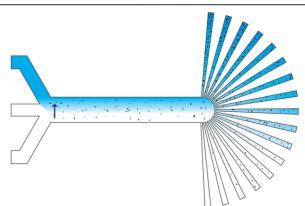
**Figure 5:** Microfluidic device to increase the concentration of bacteria by chemotaxis in different channels. Figure adapted from (27).
