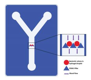
Figure 3: Microfluidic device for objective 1
